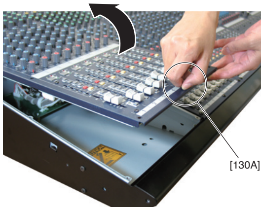
[130]: BIND HEAD SCREW-B (小ネジ+ B I N D) 4.0X16 MFZN2B3 (WE968600)
